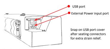
Note: Can be used with either 12V or 24V vehicle systems.
