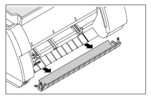
**Installing Tractor** – Raise the front cover.
