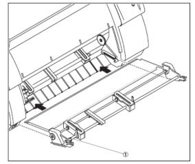
Installation must be performed with the gear on the tractor on the right side.
