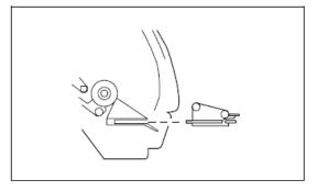
Insert the tractor with the rails on the left and right in parallel to the stop in the guides provided on the printer until they engage.
