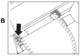
Open the colored latch lever and align the tractor so that the first printing position on the paper matches the **X** mark on the printer housing.
