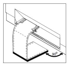
Make sure to align the paper stack in parallel with the printer and that the paper flow is unobstructed.
