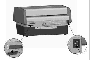
Connect the printer cable from the host computer to the printer port on the right side of the rear panel.
