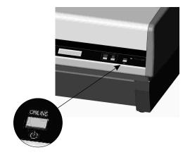
Turn the printer on by pressing the *ONLINE* button located on the front panel of the printer.
