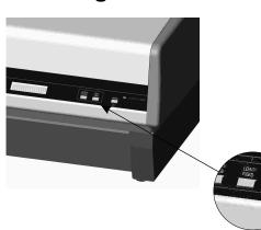
With the printer "off line", select the form you wish to print by pressing the *UNLOAD/CHANGE* button until the form name appears on the display. Press the *LOAD/FEED* button to load the form.
