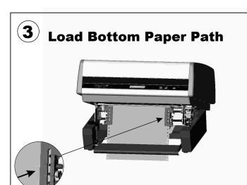
Loading paper in the bottom tractor is similar to the rear tractor. Just load paper on the 3 pins of the left and right tractors. Adjust the right tractor for paper width by releasing the green lever and sliding the tractor either to the left or right. **NOTE: The left tractor is not adjustable. Do not attempt to move it.** When done, lock the green lever back down.
