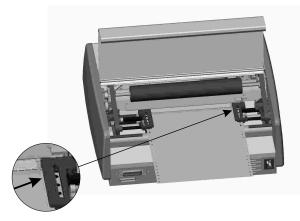
Load paper on the 3 pins of the left and right tractors. Adjust the right tractor for paper width by releasing the green lever and sliding the tractor either to the left or right. NOTE: The left tractor is not adjustable. Do not attempt to move it. When done, lock the green lever back down.
