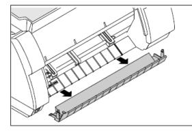
**Installing Tractor** – Raise the front cover. Remove the bottom cover.
