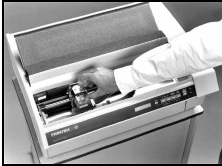
Lowering (closing) Ribbon Loading Bail
