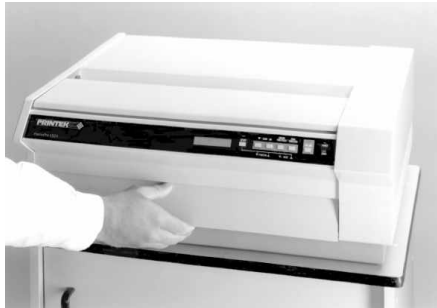
Opening The Latch Panel
