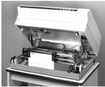
FormsPro 4503se With Forms Installed in Front Tractor Path.
