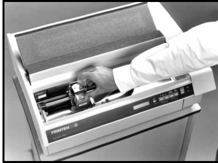
Closing the Ribbon Load Handle
